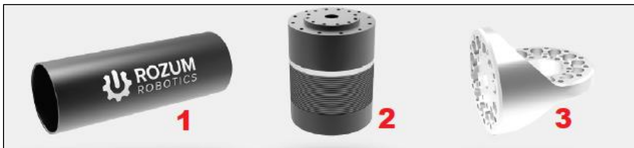
Figure 1-1: Structural elements of the PULSE robotic arm
